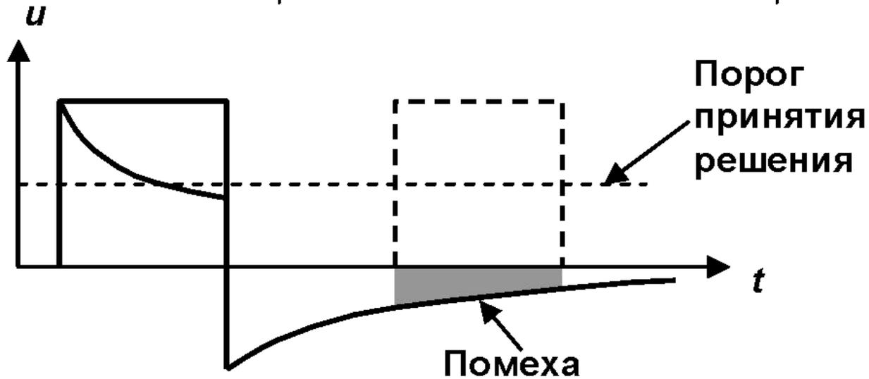
$$\tau_H = (R_c + R_H)C_p \quad \tau_H = L_1 / (R_c \parallel R_H) \quad \tau_H = 1/2\pi f_{НС}$$
