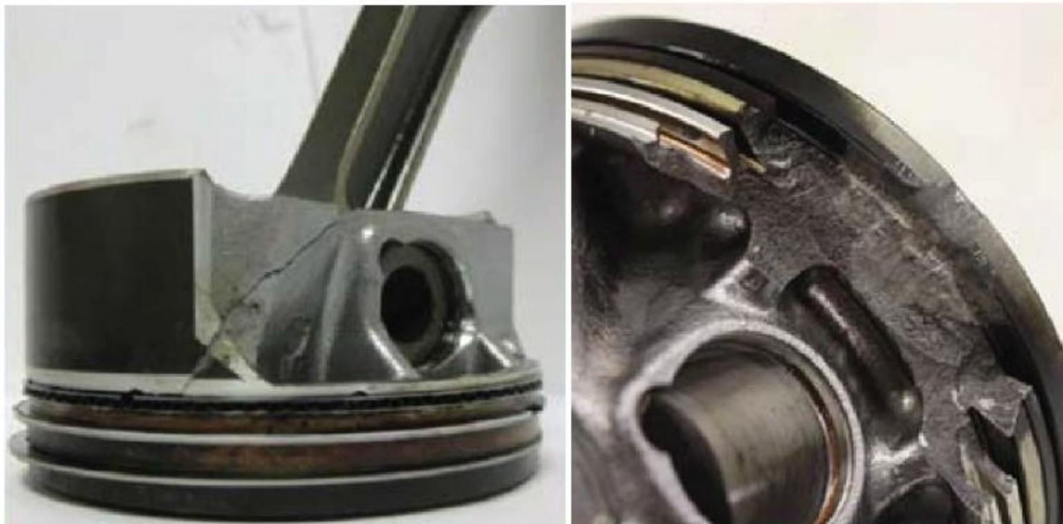
**Two examples of piston damage due to LSPI observed during testing at Southwest Research Institute<sup>®</sup>**
