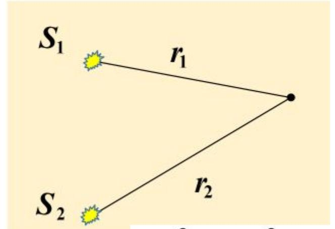
$$I = I_{max} = (A_1 + A_2)^2, \quad \cos \delta = 1, \quad \delta = 2\pi m, \quad m = 0, \pm 1, \pm 2, \dots$$
