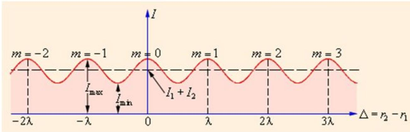
$$V = \frac{I_{max} - I_{min}}{I_{max} + I_{min}} = \frac{2\sqrt{I_1 I_2}}{I_1 + I_2}$$
