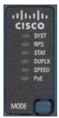
**System LED (SYST):** Shows whether the system is receiving power and functioning properly.
