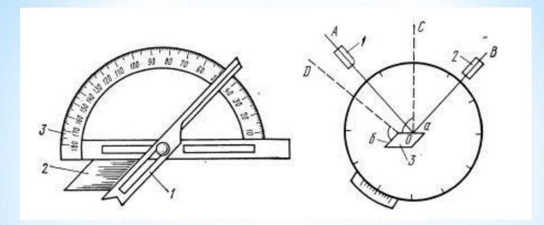
Figure 3. Applied goniometer: 1rotating ruler, 2 measured crystal, 3 protractor Figure 4. Diagram of the reflective goniometer: 1 - collimator, 2 telescope, 3 - crystal
