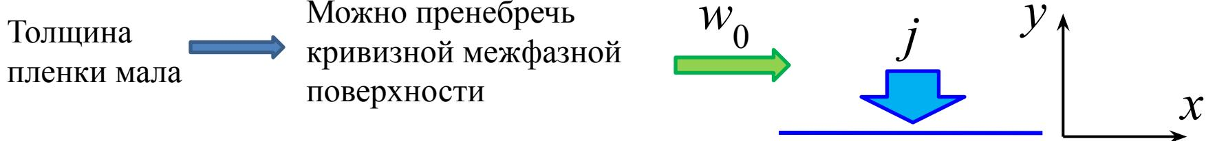
$$w_x \frac{\partial w_x}{\partial x} + w_y \frac{\partial w_x}{\partial y} = \nu \frac{\partial^2 w_x}{\partial y^2}$$
