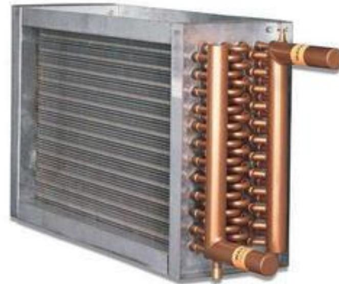
The coils are shown in dark orange in the main filter house. These are typical cooling coil construction with tubes circulating water and fins to cool the air. No particles removed in this section but the water vapor (H<sub>2</sub>O) gas is condensed in to liquid water that drains off the fins here and runs out drains under the coils.
