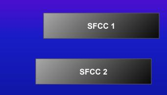
The slats and flaps are hydraulically actuated like all the other surfaces. They are electrically controlled via two Slat Flap Control Computers (SFCC).
