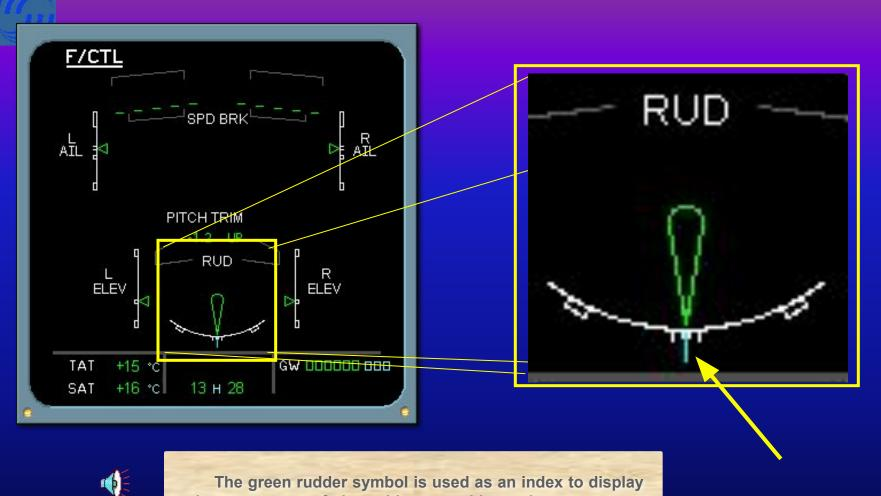
The green rudder symbol is used as an index to display the movements of the rudder on a white scale.
