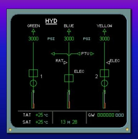
Three independent hydraulic systems are used to power all the flight control surfaces.
