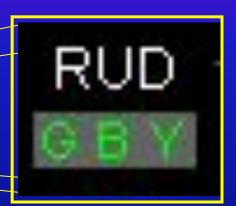
The hydraulic systems which actuate each control surface are indicated on the ECAM F/CTL page by the use of G, B and Y.
