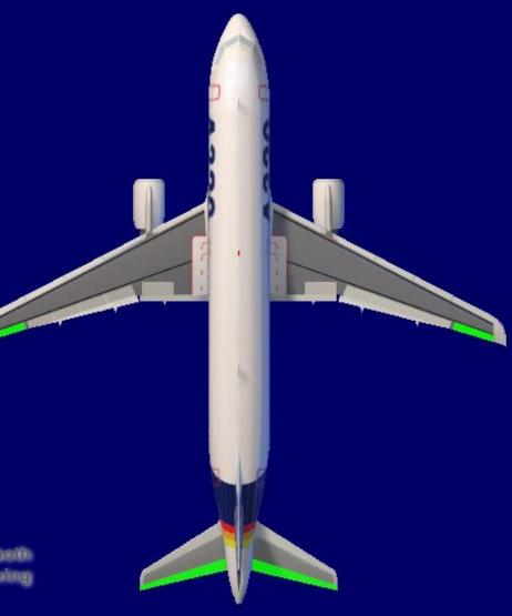
The movements of both ailerons and both elevators are symbolized by a green index moving in front of a white scale.
