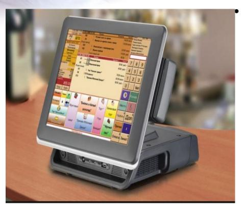
R-keeper supports TCP / IP network protocols. The system involves the installation of special kitchen monitors, devices to call the waiters, and printing checks.
