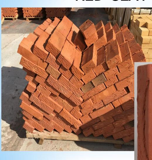
Red clay bricks are made from clay mixed with water, followed by molding, drying and firing.
